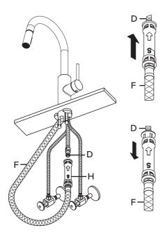
Attach Quick Connect (H) with black end onto spray hose (F) until you hear a click. Attach the other end onto the supply hose (D) until you hear a click.
