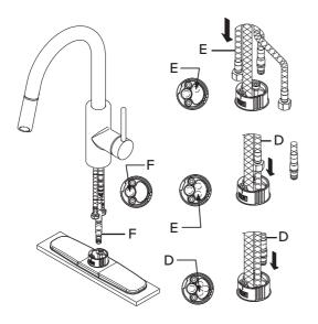
Remove Quick Connect (H) from spray hose (F). Insert spray hose (F) into small hole of base (J). Insert hot & cold waterlines(E) and supply hose (D), one by one, in large hole of base
