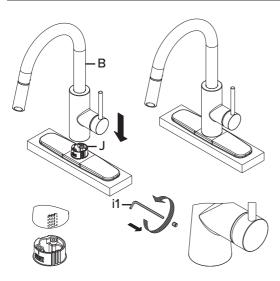
**Note:** "▲" on base should be in alignment with "▼" on faucet body.
