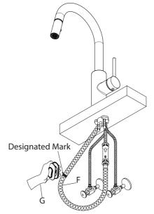
Attach weight (G) on the designated mark on the spray hose (F)
